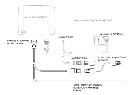
Figure 5-2. In Cab Weather Station Layout
